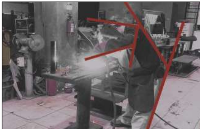
Figure 3. Welding posture during the welding process after being identified
