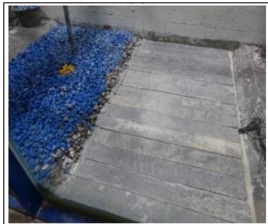
Figure 3. Testing on flexible pad + rock compound
