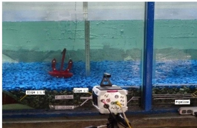
Figure 4. Image of the anchor falling on the protection layer
