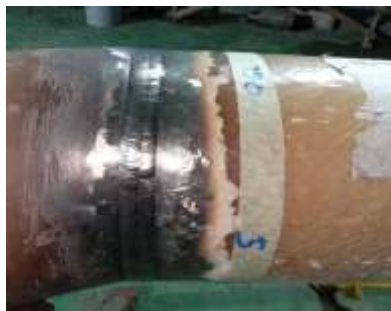
Figure 3 Surface results of welding sections 0-5 inch
