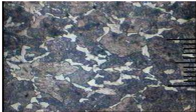
Figure 6. Structure Micro Test results preheating 300°C on ST60 steel [6]
