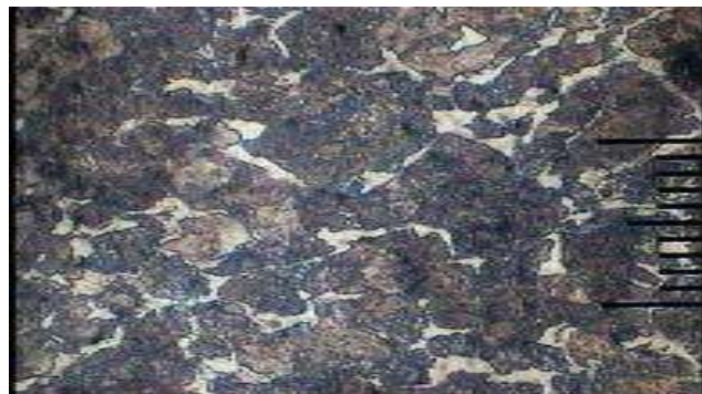
Figure 7. Structure-Micro Test results Preheating 400°C on ST60 steel [6]
